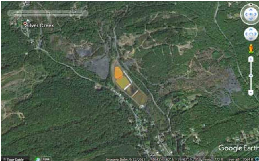
The Silver Creek acid mine drainage treatment system is a passive system that does not require electricity or pumping to cleanse the water as it flows from the first pond (top) to the outfall (bottom) through a series of ponds.
